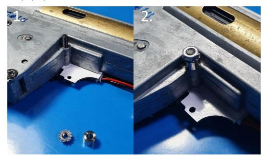
5. Use two 8 mm screws and nuts to secure the front of the gearbox.
