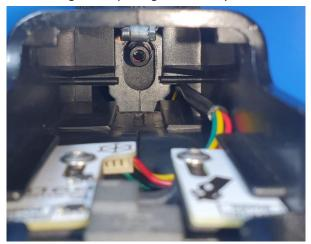
8. Install the back plate and fasten the control board to it. Use provided 12 mm screws.
