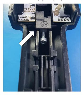
10. Install the trigger board, control board, and the holding piece in the receiver as shown on photo below.
